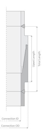
1. Matched Strength (MS): The coupling OD is adjusted to the minimum critical area capable of providing the same tensile efficiency as the pin end, allowing better clearance<sup>1</sup>.
